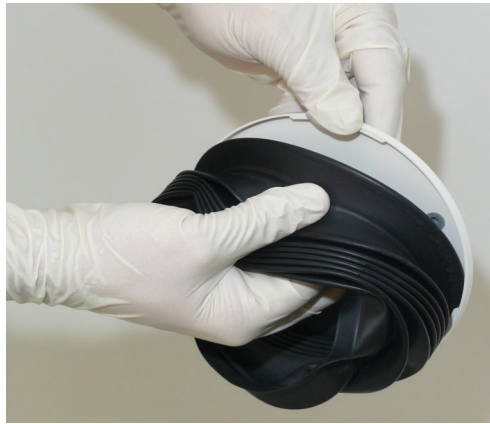
FIGURE 7-7 Detaching the Bellows Top Plate
