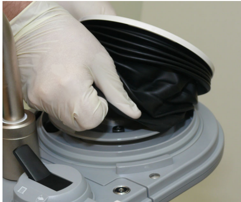
FIGURE 7-6 Detaching the Bellows
