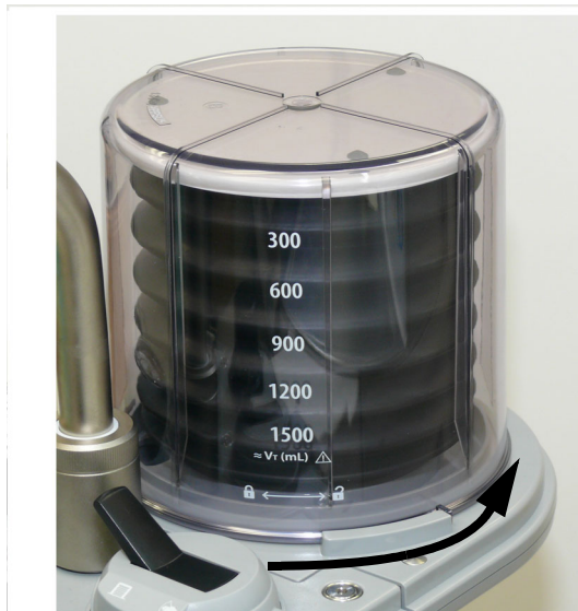
FIGURE 7-5 Removing the Bellows Dome
