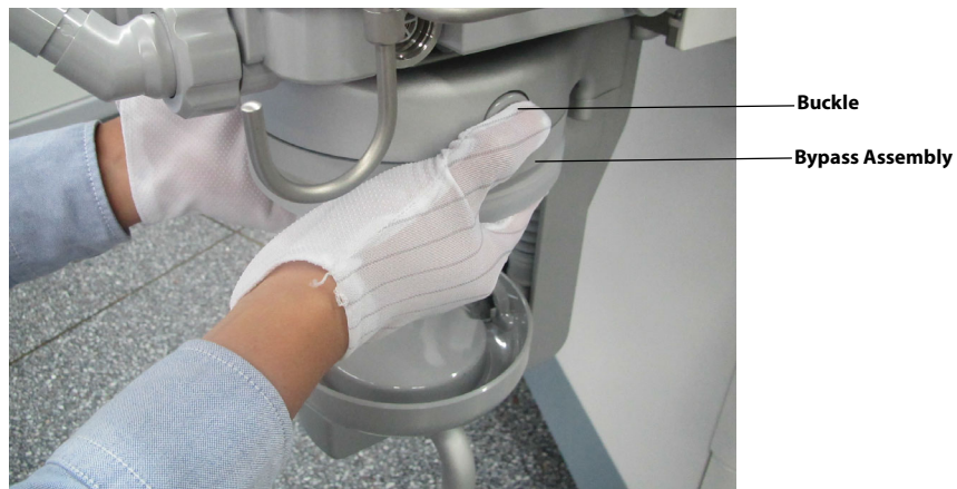
FIGURE 7-22 Remove Bypass Assembly
