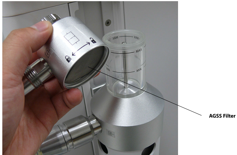
FIGURE 7-27 Removal of AGSS Top / AGSS Filter Inspection
