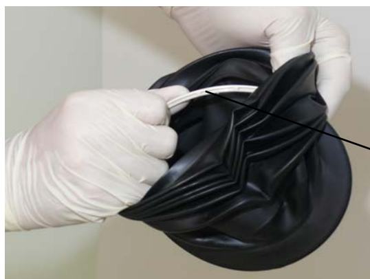
FIGURE 7-8 Removing the Bellows Adapter Ring
