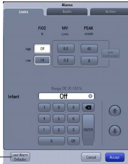
FIGURE 6-10 Load Alarm Defaults button in the Alarms window (without AG module connected)
