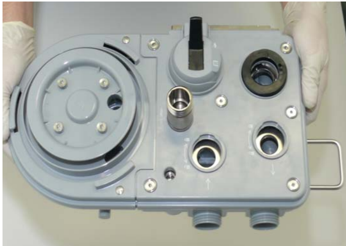
FIGURE 7-24 Breathing System Block Removal, Top View
