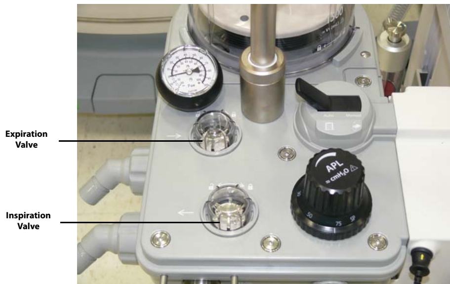
FIGURE 7-10 Location of Expiration and Inspiration Valves
