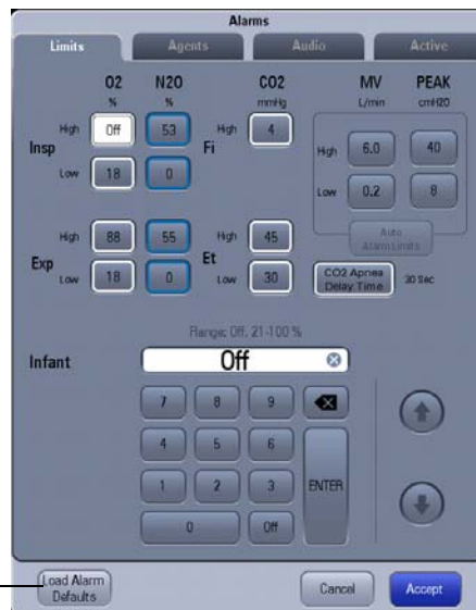
FIGURE 6-11 Load Alarm Defaults button in the Alarms window (with AG module connected)
