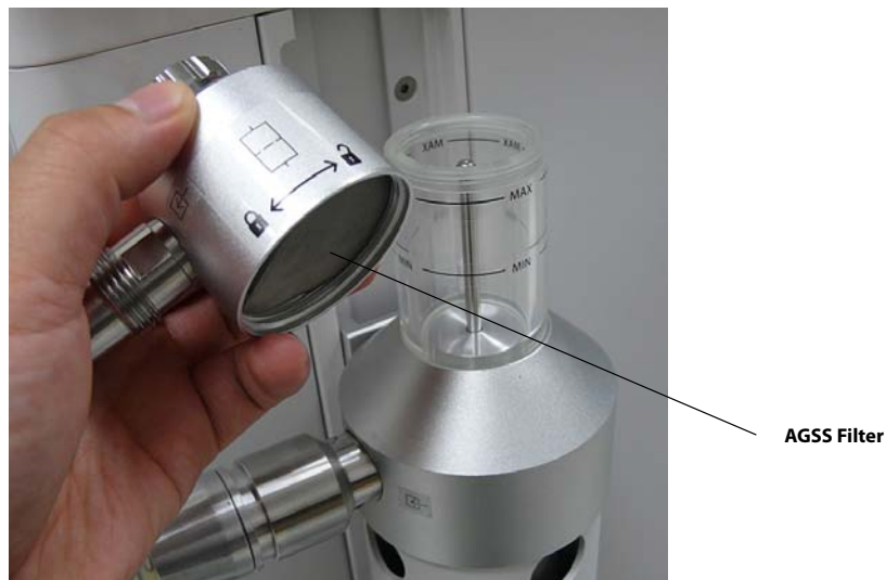
FIGURE 7-27 Removal of AGSS Top / AGSS Filter Inspection
