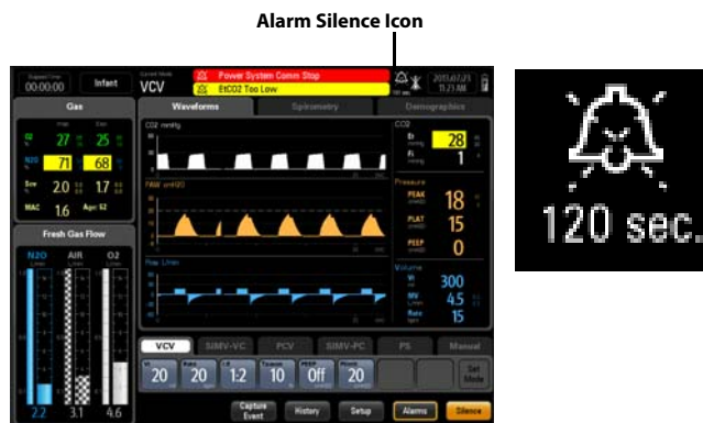
FIGURE 3-9 Alarm Silence Icon (with AG module connected)
