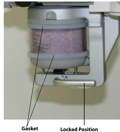
FIGURE 7-20 Absorber Canister, Locked
