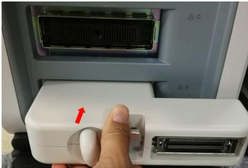
2. Move the probe adapter locking lever to horizontal position through 90° clockwise and lock it.
