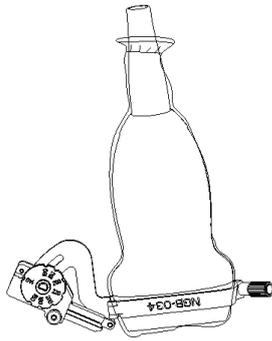
4. Adjust the dial scale to the required needle type shift.
