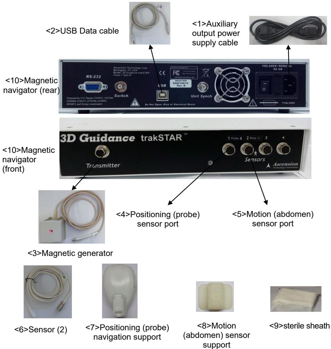
The description of the magnetic navigator is given in details. See the table below.
