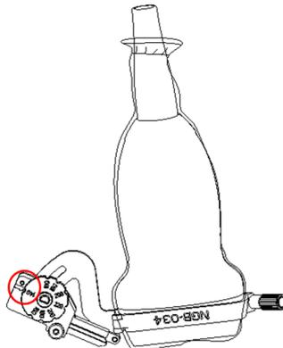
5. Adjust the needle angle to the proper shift as required (loosen the nut first, and then tighten the nut based on the shift you need).
