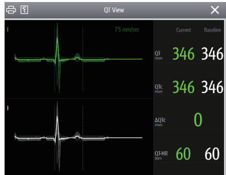
Figure 9. QT View provides baseline and current ECG for comparison
